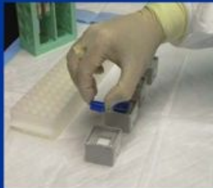
Remove and discard pre-filter
